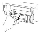
**3** Set the AIT data cartridge orientation as shown here and insert it into the data cartridge slot.
